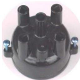
It is possible for all components of the distributor to be functioning but still have a negative effect on the running of the engine. The power can be there and have all connections properly in place and yet have a defective or cracked **distributor cap**. Such a covering can short circuit the distributor; it can not be repaired so it must be replaced.
